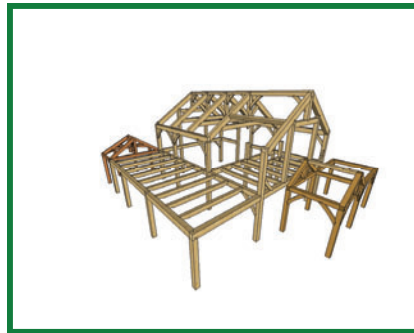
Pictured left: CAD drawing of the Sass frame, highlighting three species of hardwoods incorporated.
